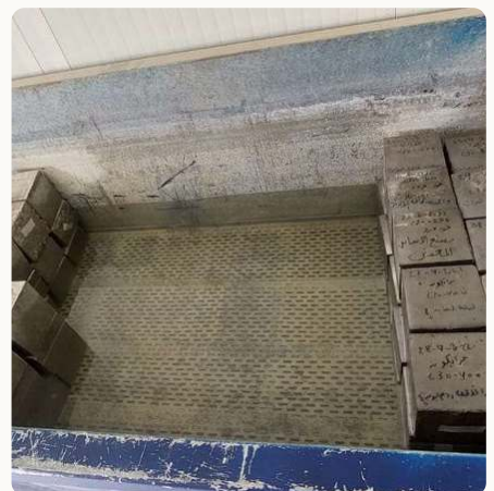
Concrete cube curing tank
